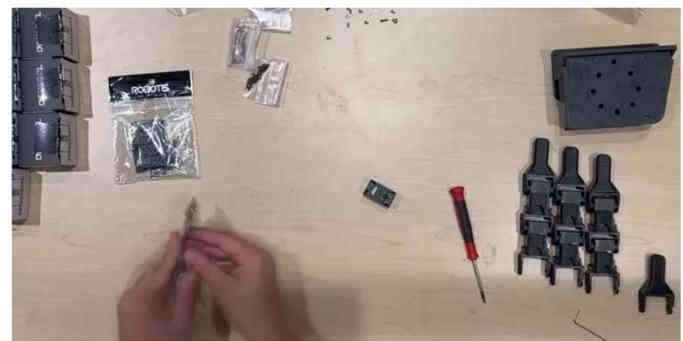
LEAP Hand can be built in under 3 hours using a 3D printer, off-the-shelf parts and 3 hand tools.
